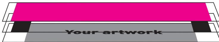
The white SPOT layer (marked as magenta) is placed in the top layer, as the artwork is printed mirrored on the transparent polycarbonate sheet.
